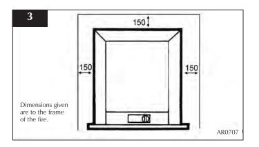
2.8 The maximum depth of combustible shelf is 150mm at a minimum height of 150mm above the frame.
